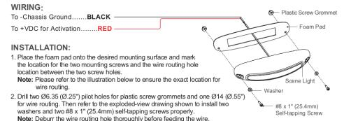
Feed the wires through the foam pad and wire routing hole and mount the scene light with the supplied self-tapping screws.
