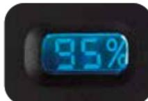
When the searchlight is turned **ON** the digital battery display will show the % of battery capacity.
